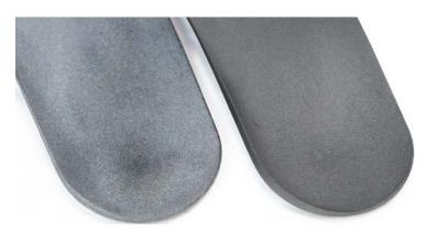
Figure 6. Printed part cleaned with glass beads (left); part cleaned with metal media (right)
