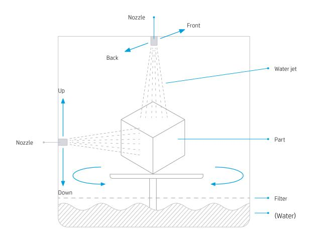
Figure 8. Water jet blasting equipment
