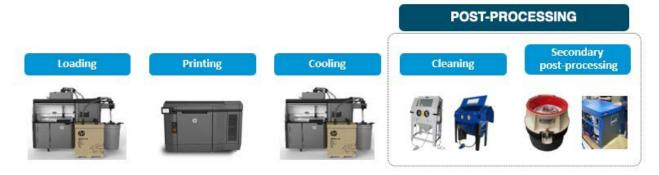
Figure 1. E2E HP Jet Fusion 3D Printing workflow
