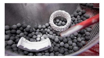
Figure 4. Automatic bead blaster
